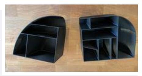
with the radius of curve and redesigned the front. I printed this without support and at a later height of .24, it 'only' took 27 hours.
