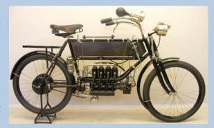
starter (the rider pedalled a chain drive and sprockets to turn the rear wheel) it had 'modern' high-tension Bosch magneto ignition and a spray carburettor. Earlier models had a rear coaster brake operated by the pedals but by 1909 a rear drum brake was fitted. By 1911/12 it was the world's fastest production motorcycle at 40 miles per hour.
